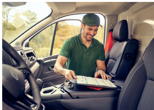
Fold-down centre backrest provides a stable and convenient work surface
